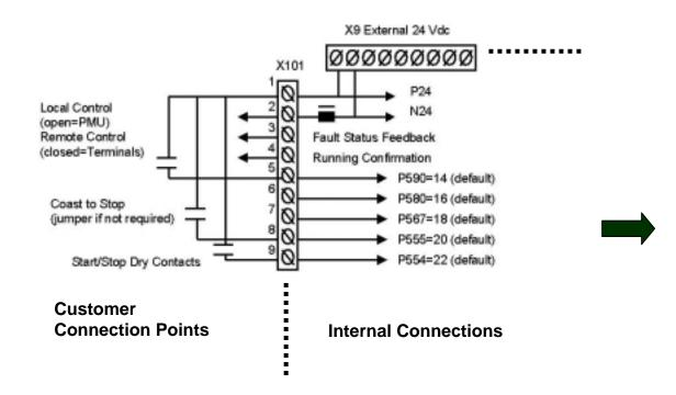
Step 1: Dry set of contacts between terminals X101, pin#1 and pin#5 for Local/Remote Mode Selection. Jumper if not required.
